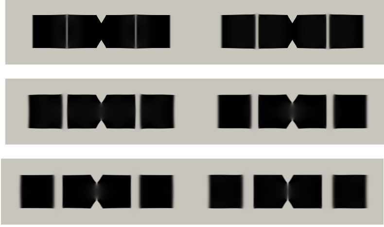
Figure 5.7: The plate breaking dynamics is shown for V = \pm 100 \text{ m/s} for time instants 1.4 \times 10^{-3} \text{ s} , 2.7 \times 10^{-3} \text{ s} , 4.0 \times 10^{-3} \text{ s} , 5.4 \times 10^{-3} \text{ s} , 6.7 \times 10^{-3} \text{ s} and 8.3 \times 10^{-3} \text{ s}
