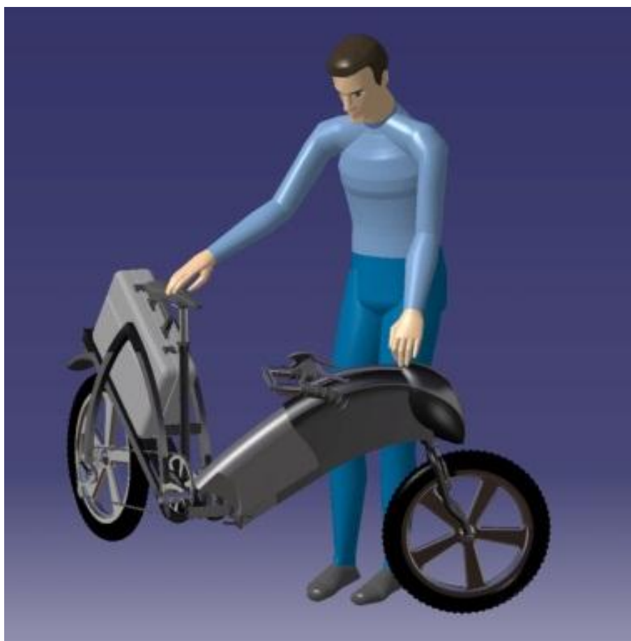
Figure 45 - Phase de pliage du vélo (4/4)
