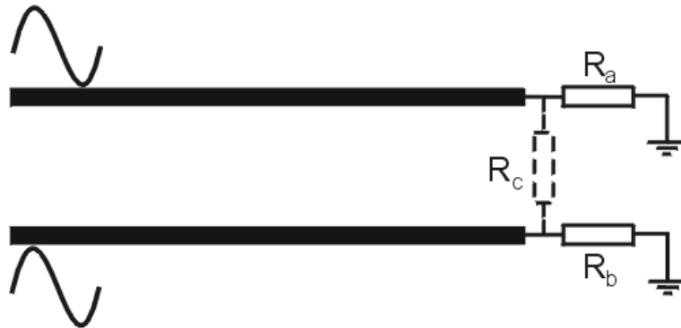
Equivalent termination in Even mode
