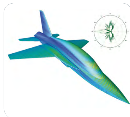
Simulation of Radar Cross Section of a jet fighter airplane at 3GHz with Efield® MLFMM with more than 106 unknowns
